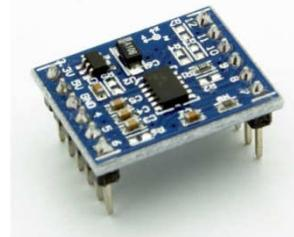
Gambar 3 Modul Sensor Akselerometer MMA7361L
