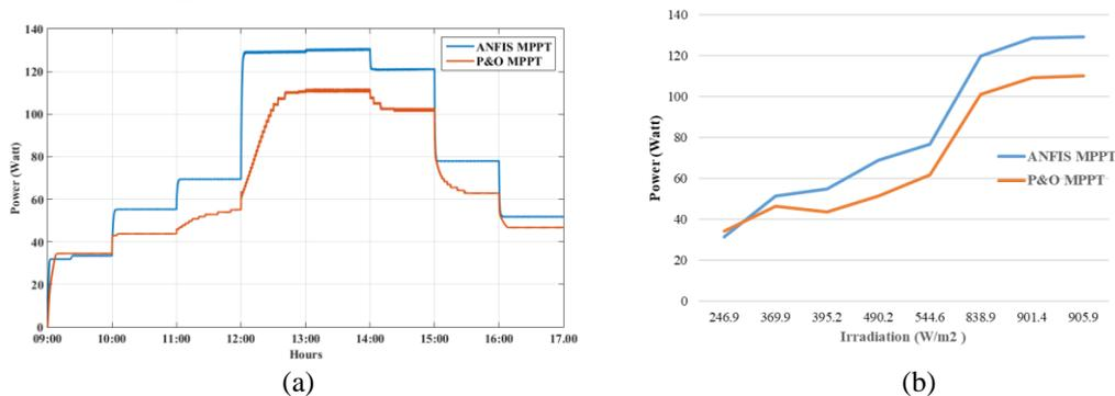
**Fig. 7.** ANFIS MPPT vs. P&O output power of boost converter on Saturday, September 4, 2021: (a) Hourly output power; (b) Output power trend due to irradiation
