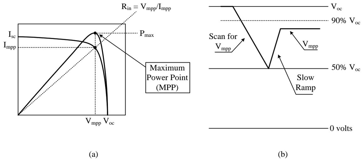
**Fig. 2.** MPPT for photovoltaic: (a) MPPT versus photovoltaic curve; (b) MPPT scanning operations
