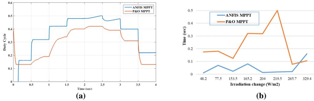
**Fig. 8.** ANFIS MPPT vs. P&O transient time on Sunday, September 5, 2021: (a) Transient time every change of duty cycle; (b) Transient time trend due to irradiation change
