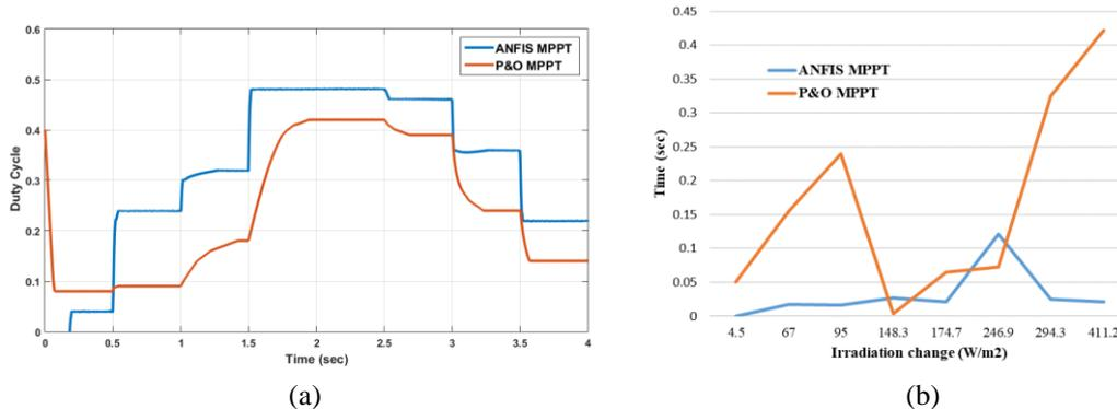
**Fig. 6.** ANFIS MPPT vs. P&O transient time on Saturday, September 4, 2021: (a) Transient time every change of duty cycle; (b) Transient time trend due to irradiation change
