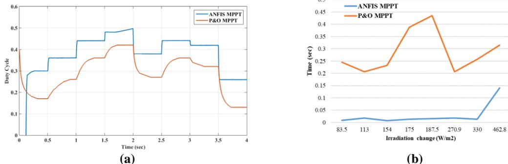
**Fig. 10.** ANFIS MPPT vs. P&O transient time on Monday, September 6, 2021: (a) Transient time every change of duty cycle; (b) Transient time trend due to irradiation change
