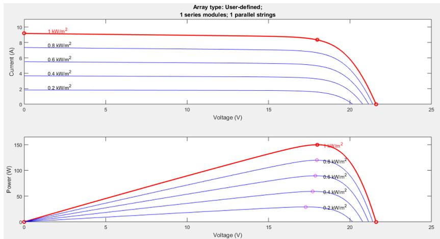
**Fig. 5.** Characteristic curve of the Solarimba SRB150M photovoltaic module
