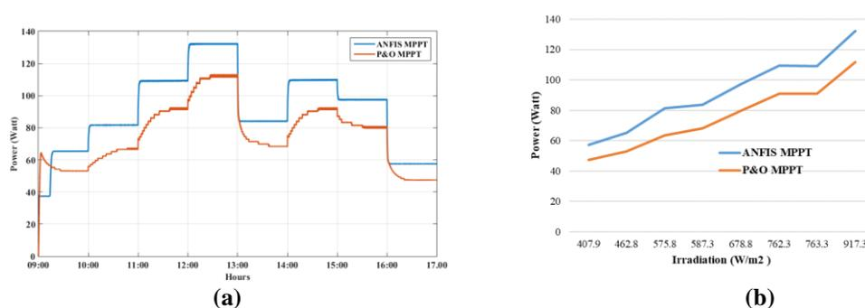
**Fig. 11.** ANFIS MPPT vs P&O output power of boost converter on Monday, September 6, 2021: (a) Hourly output power; (b) Output power trend due to irradiation
