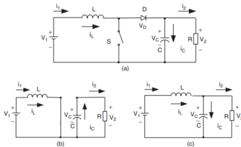
**Fig. 1.** Boost converter: (a) circuit diagram; (b) switch-on equivalent circuit; and (c) switch-off equivalent circuit.
