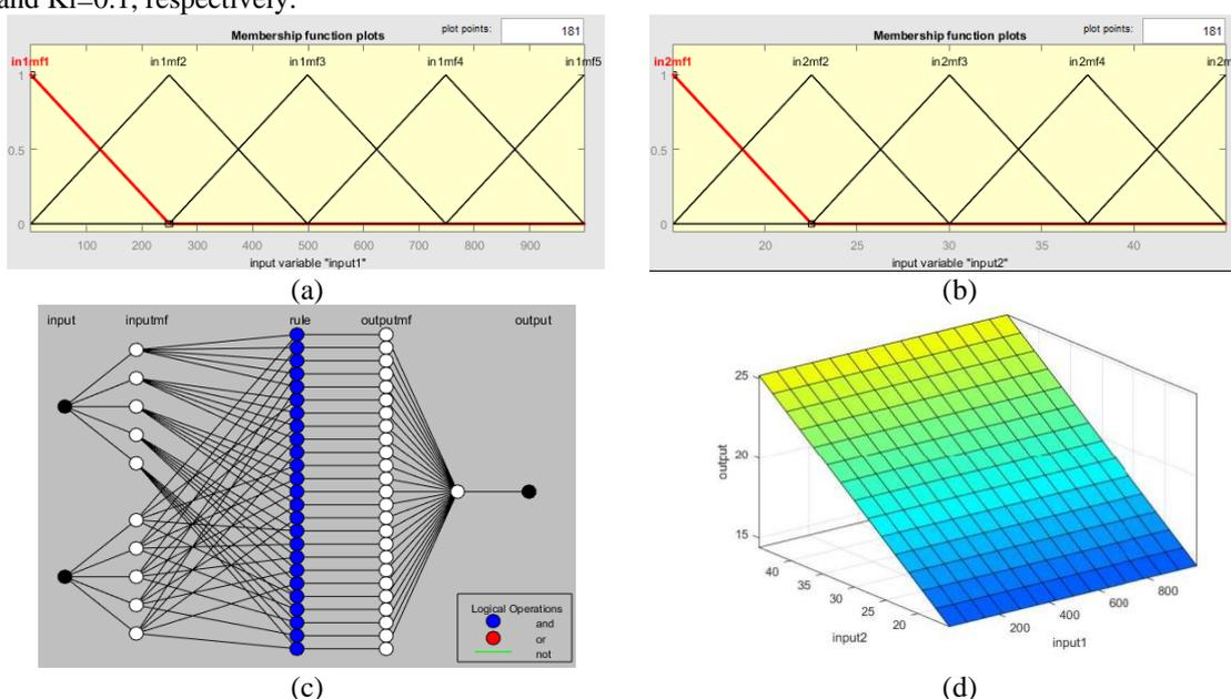
**Fig. 4.** ANFIS-based MPPT controller training results: (a) membership functions of irradiation; (b) membership functions of temperature; (c) structure; (d) I/O surface
