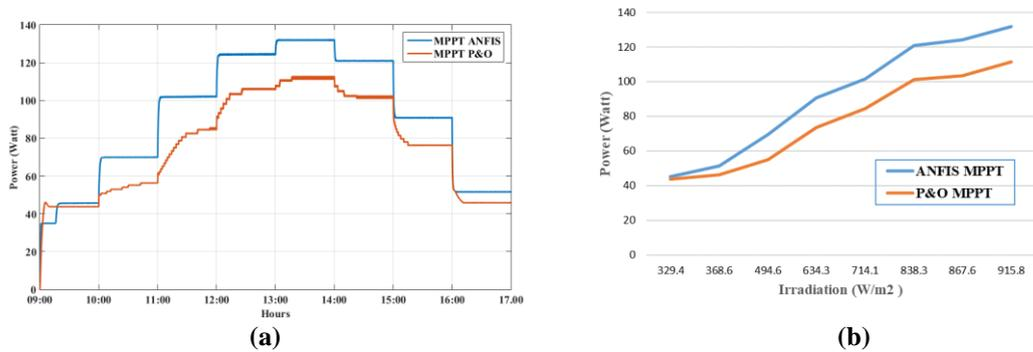
**Fig. 9.** ANFIS MPPT vs. P&O output power of boost converter on Sunday, September 5, 2021: (a) Hourly output power; (b) Output power trend due to irradiation
