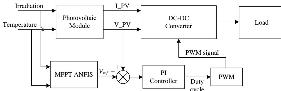
**Fig. 3.** Photovoltaic system design with ANFIS-based MPPT controller
