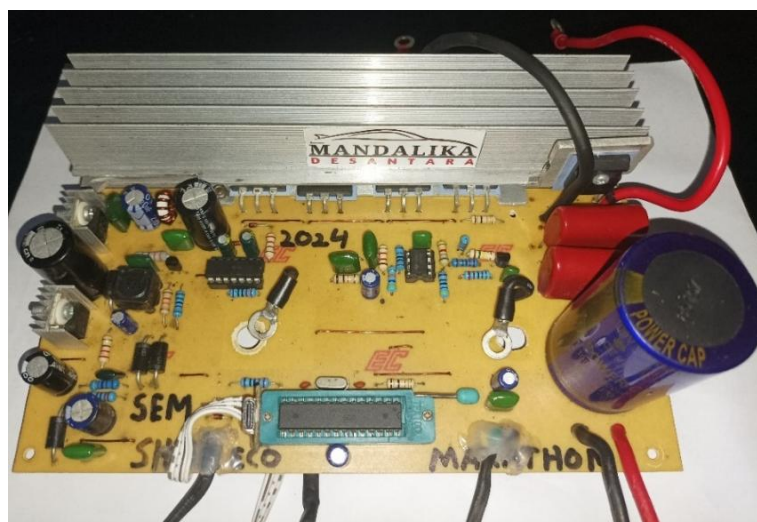
Gambar 4. (a)Power Supply (Buck Converter), (b)Gate Drive, (a)Minimum sistem ATmega328P
